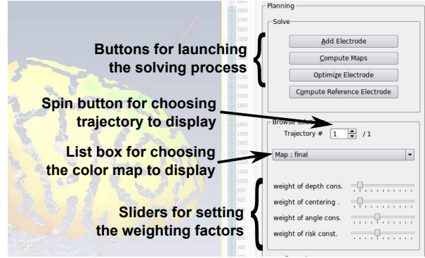
FIGURE 7.8: Snapshot of our software, showing the interface allowing to modify the settings, to change the color map to display, and to browse the proposed optimal trajectories if several are found
